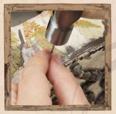
**1. PREPARE FOR A HOLE** To wire two objects together, sometimes it's necessary to drill a hole in one or both objects. Here, I want to drill a hole into this metal box, but before I actually drill, I make a small dent in the metal, using a hammer and a nail. This will keep the drill from "walking."
