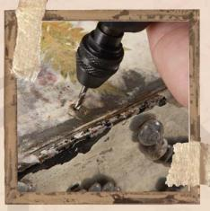
2. DRILL THE HOLE Now it's a snap to drill the hole. Just place the drill bit in the indention and drill.
